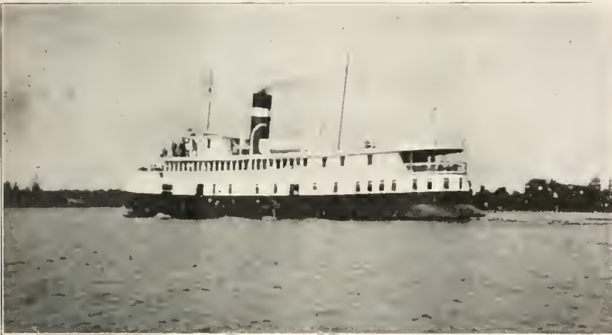
Boats plying upon the waters adjacent to summer resorts are required to provide tankage for their sewage, in which the contents are subjected to sterilizing treatment by live steam for one hour and then dumped at a safe distance from any wharf or place of residence.
